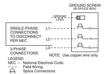
Fig. 17 - Line Power Connections
